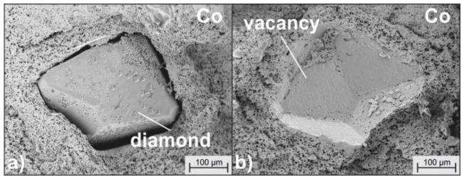
Fig. 9: Fractured surfaces of thermally post-treated Co-based diamond segments
