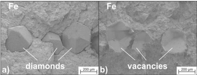
Fig. 2: Fractured surfaces of hot-pressed Fe-based diamond segments
