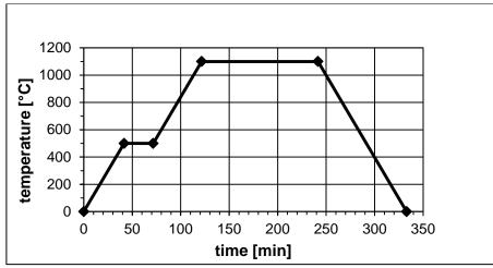
Fig. 1: Heating process of the post-treatment
