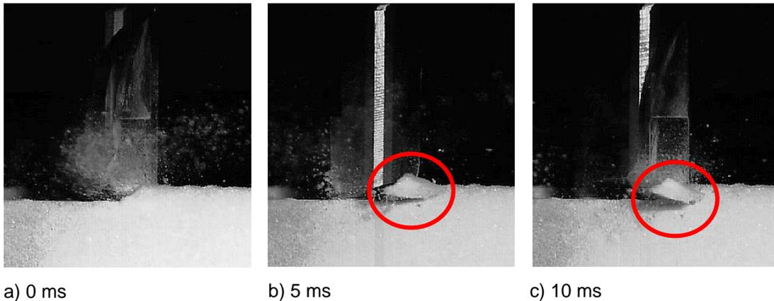
Fig. 6: Snapshots of the machining of Carrara Marble
