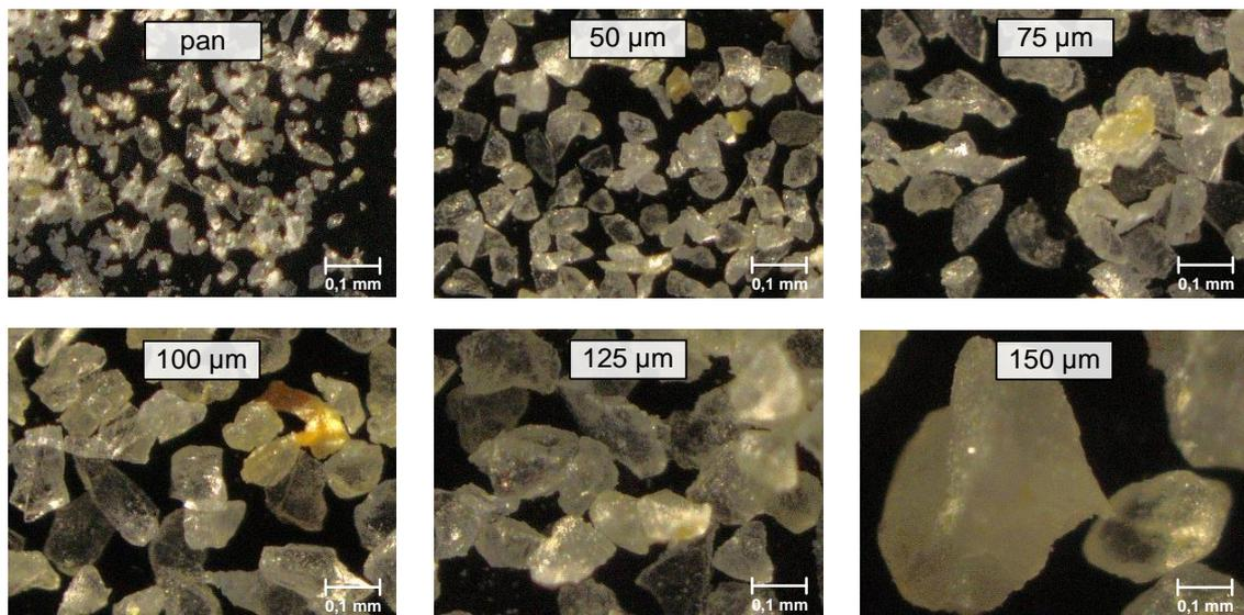
Fig. 2: Particle distribution for Postaer Sandstone
