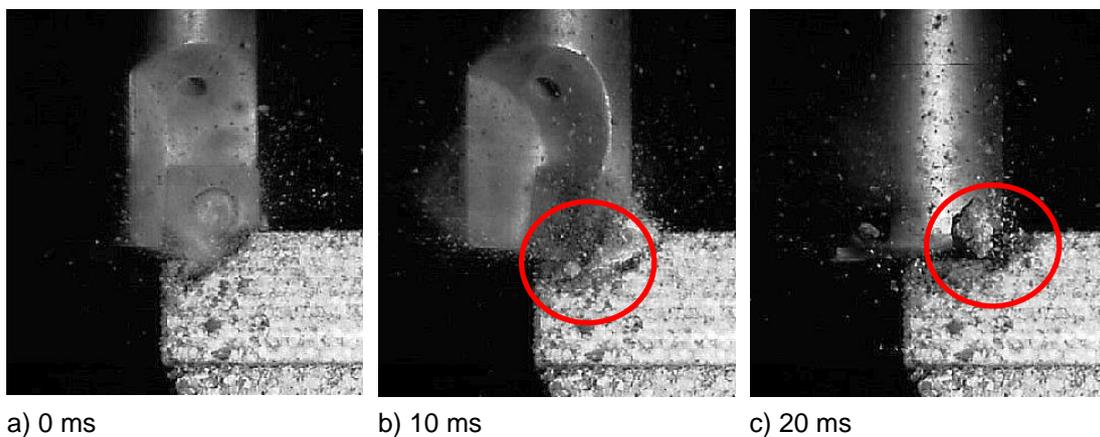
Fig. 5: Snapshots of the machining of Postaer Sandstone
