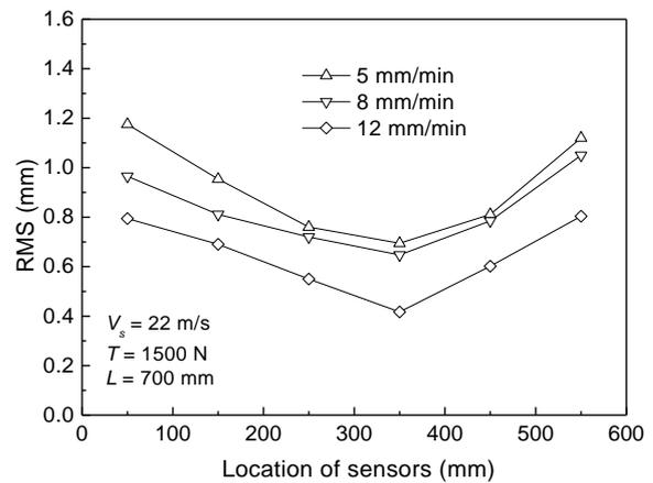
Fig. 5 Effect of the wire speed on wire amplitude
