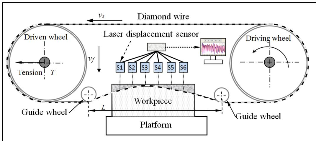
Fig. 3 Illustration of the wire vibration measurement
