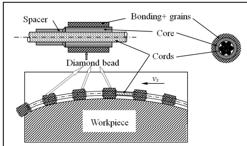
Fig. 1: Illustration of the diamond wire sawing
