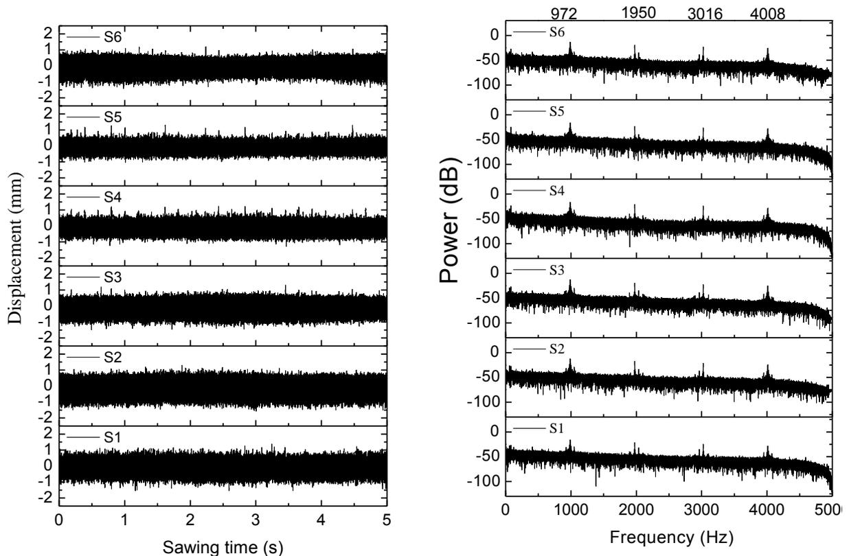
(a) Typical vibrations at different measurement points (b) FFT curves of vibration signal
