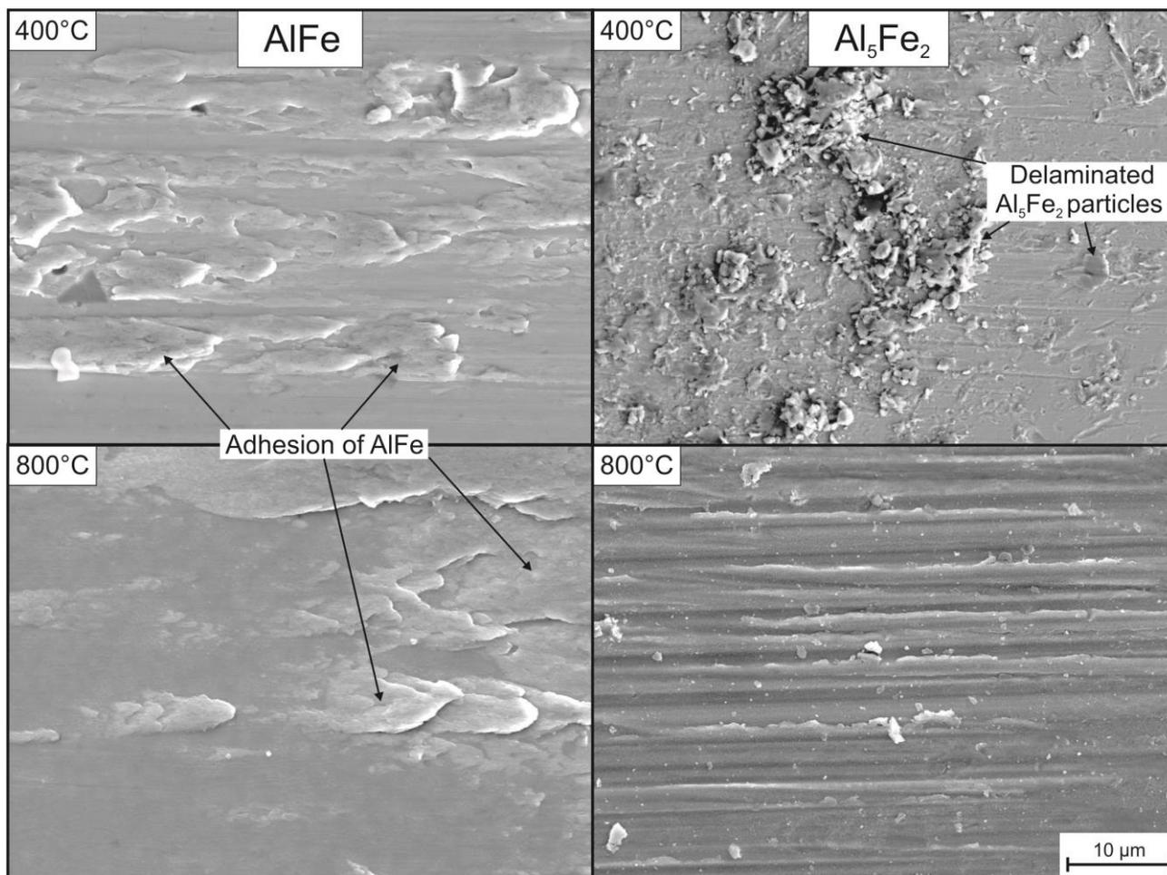
**Fig. 3:** SEM micrographs of the X38CrMoV5-3 hot-work tool steel worn surfaces after wear tests against AlFe and Al<sub>5</sub>Fe<sub>2</sub> at 400°C and 800°C.
