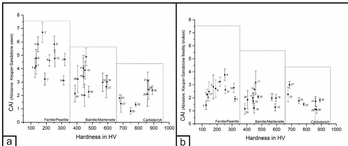
**Figure 5.** CAI value against hardness of the test body for the abrasive Keuper-sandstone with a) sawn and b) freshly broken surface. The used materials are grouped referring to their microstructure. The numbering denotes the relevant test body material and heat treatment state (Tab. 1).
