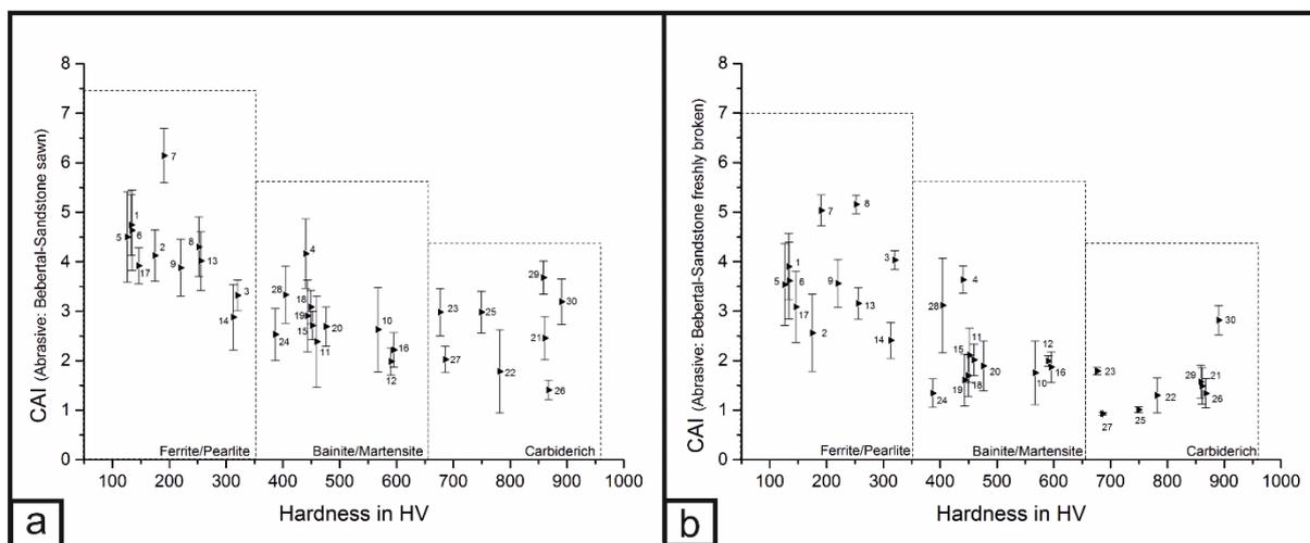
**Figure 6.** CAI value against hardness of the specimen for the abrasive Bebertal-sandstone with a) sawn and b) freshly broken surface. The used materials are grouped referring to their microstructure. The numbering denotes the relevant test body material and heat treatment state (Tab. 1).
