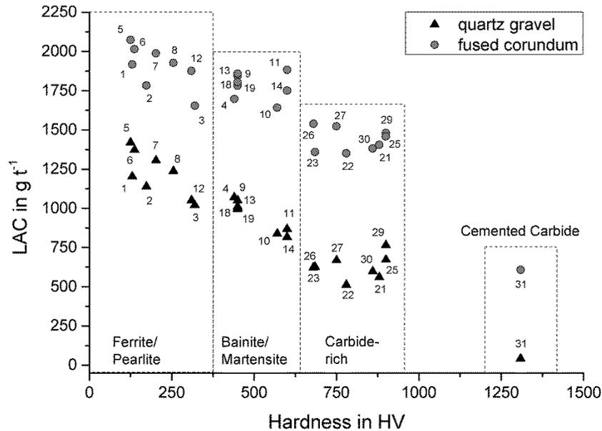
**Figure 4.** LAC value against hardness of the impeller for the abrasives crushed quartz gravel and fused corundum. The used materials are grouped referring to their microstructure. The numbering denotes the relevant impeller material and heat treatment state (Tab. 1).
