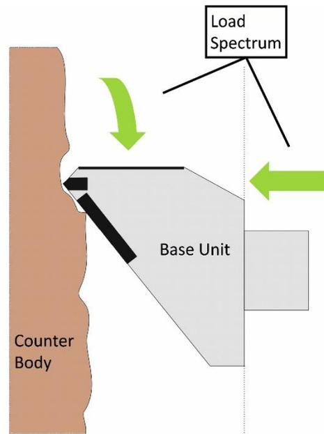
**Figure 7.** Tribological system for a TBM tool in soil. The tool (base unit) scratches over the tunnel face/geology (counter body) and excavates the soil. This degradation process and the correlated wear of the tool are strongly dependent on the load spectrum of the tunneling process (e.g. advance rate, penetration, rotational speed).
