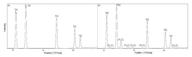
Figure 2: Phase analysis of RecyTiC-MMC-1 (a) and RecyTiC-MMC-2 (b).
