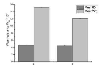
Figure 7: Wear resistance of MMC-2 (a) and MMC-R2 (b) in heat treated state.
