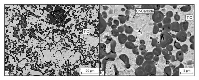
*Figure 1: Microstructure of the sample MMC-1 (a)) in solution annealed state and sample MMC-2 (b)) in soft-annealed state.*
