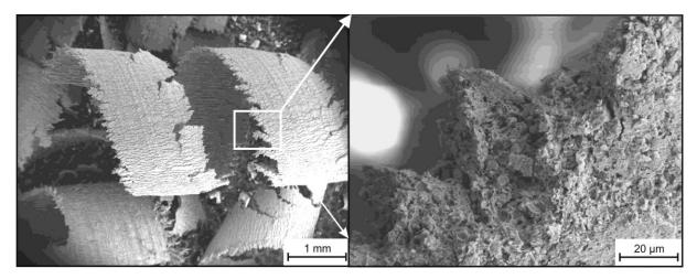
*Figure 4:* SEM Picture of the chip material used for the recycling process.
