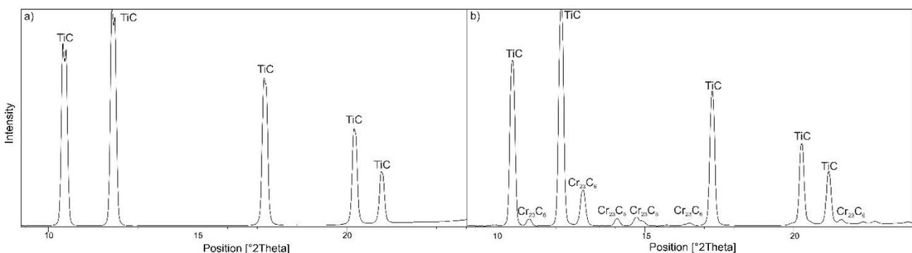
**Figure 2:** Phase analysis of RecyTiC-MMC-1 (a) and RecyTiC-MMC-2 (b).
