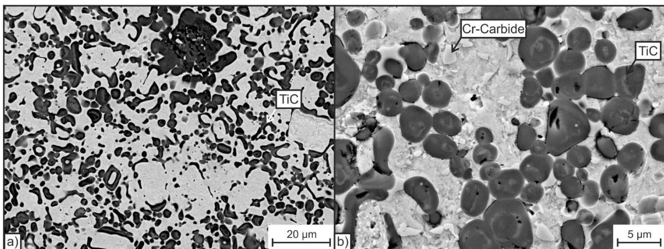
**Figure 1:** Microstructure of the sample MMC-1 (a) in solution annealed state and sample MMC-2 (b) in soft-annealed state.
