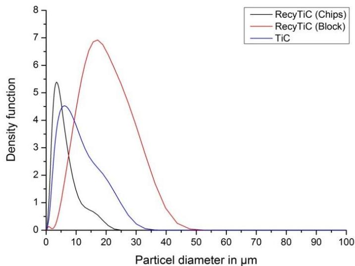
**Figure 3:** Particle size of the RecyTiC respectively TiC depending of the machining grade.
