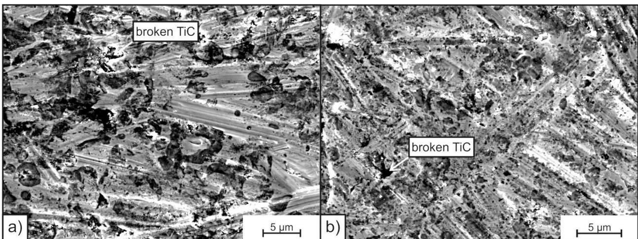
**Figure 8:** Worn surface of the material MMC-2 (a) and MMC-R2 (b) in heat treated state.
