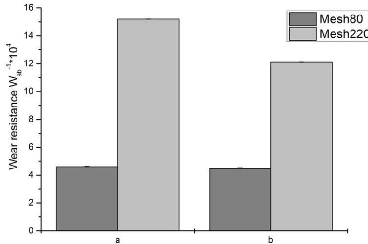
**Figure 7:** Wear resistance of MMC-2 (a) and MMC-R2 (b) in heat treated state.
