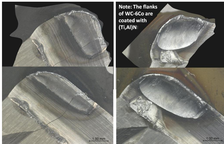
Figure 9 Comparison of crater wear in hard turning of NbC-8Co SPS (left) and WC-6Co (right) (100Cr6 (205 HB), machining time= 5 min. 33 s., V_c = 100 m/min, f = 0,415 mm/rev, hex = 0,4 , DoC = 3 mm, Kr (lead angle) = 75^\circ , nose radius= 1,5 mm, emulsion 10 bars) [10]
