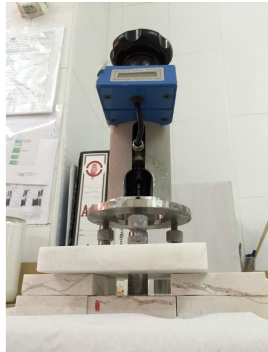
Fig. 1 and 2: Drop Angle measurement equipment (left) and adhesion strength measurement equipment and dolly – sample assembly (right).
