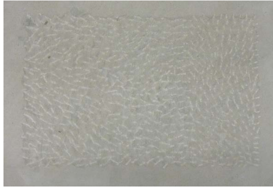
Figure 3: Line punching on a sandstone surface
