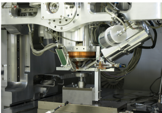
Fig. 1: Set-up with tribometer in a large-chamber SEM
