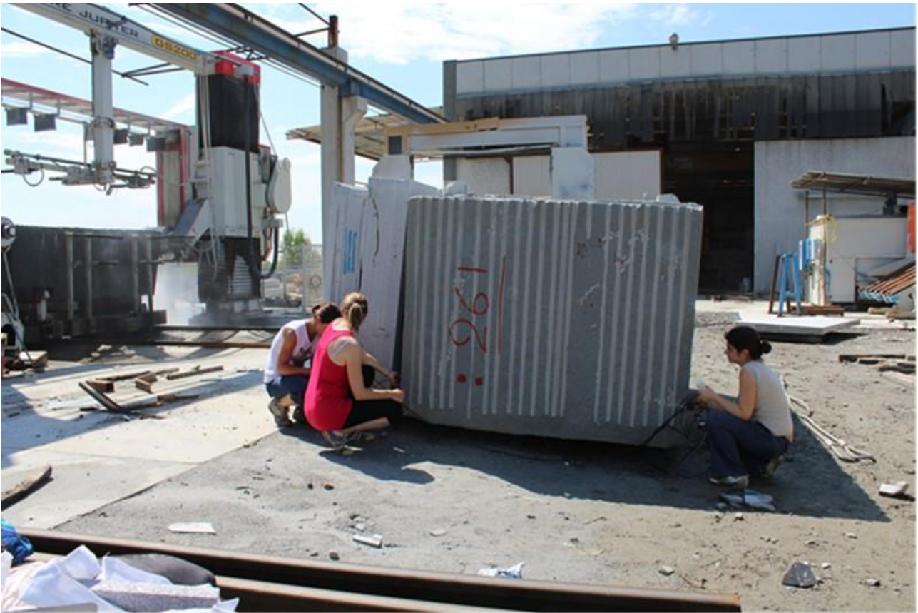
Fig 1 – ultrasonic measurements by direct method on DIOs block
