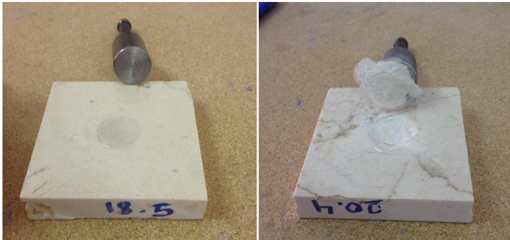
Fig. 3 and 4: Specimens showing a 100% adhesive failure (A/B) on the left and a 100 % substrate cohesive failure (A) on the right.
