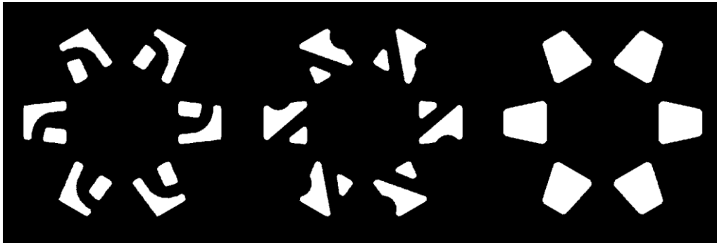
Fig. 6. Simulated polishing tools, formed by six Frankfurt abrasives: 320TX (left), 400T (center) and 5Extra (right).
