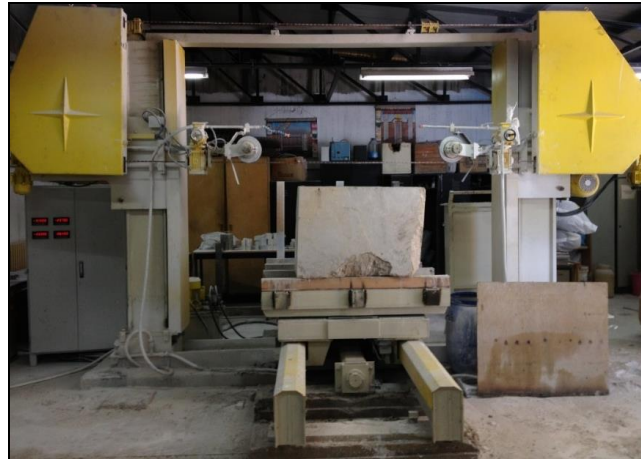
Fig. 1 General view of the mono-wire block cutting machine.
